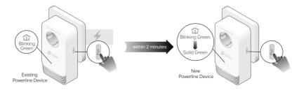
**4.** When the Powerline LED turns solid green, it's done. Relocate the new powerline adapter to the place where wired internet access is needed.
